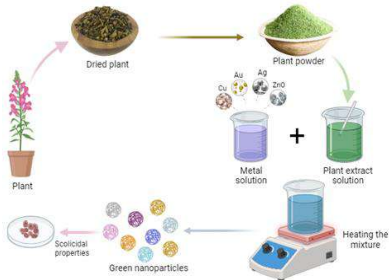
Fig. 3: Presents a potential method for synthesizing nanoparticles by using Plants (Green nanoparticle)
