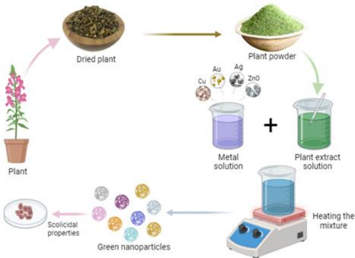
Fig. 3: Presents a potential method for synthesizing nanoparticles by using Plants (Green nanoparticle)
