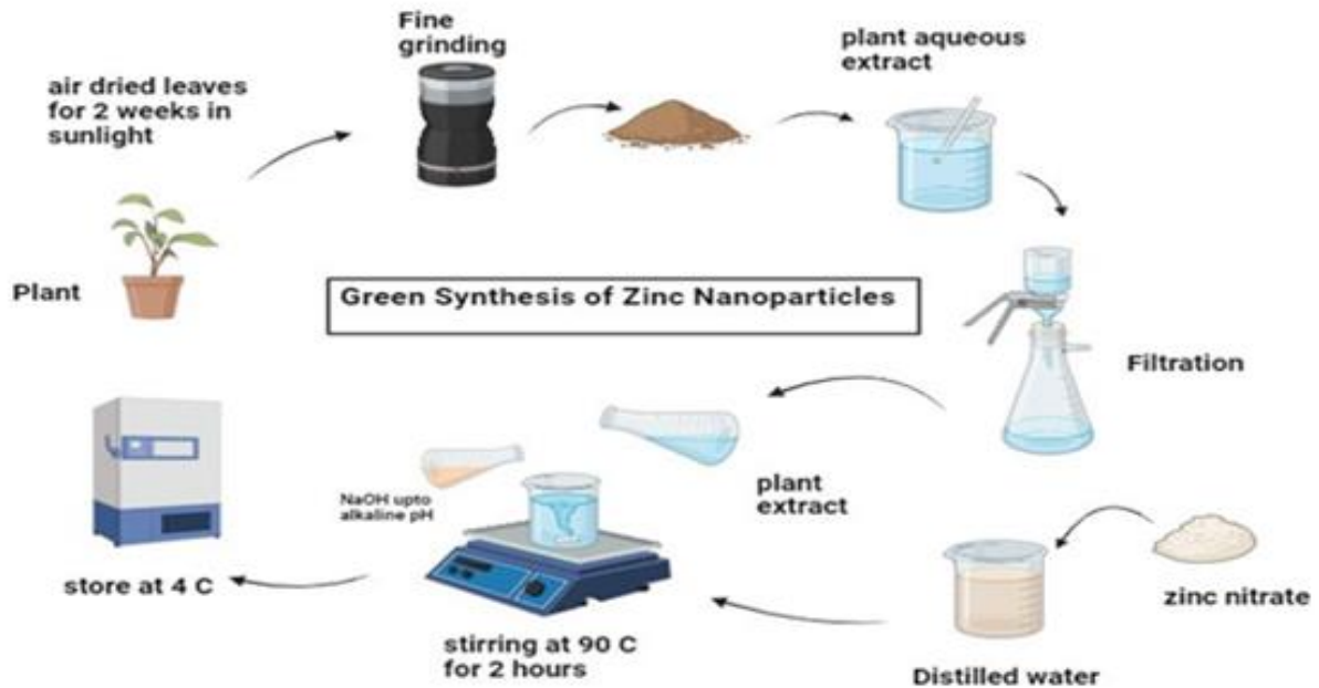
Fig.1: Biological synthesis of zinc oxide nanoparticles.
